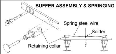
coupling hook shank once you are happy that the buffers spring freely. You can now fit the brake yokes, parts 21, by springing them between the brake blocks.
