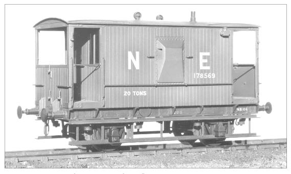
The Toad E was the final design of 10'6" wheelbase brake van built by the LNER in large numbers in the early 1930's. They remained a common sight at the end of freight trains into the 1960's.
