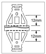
the offending hole into an oval shape until its edge is 12mm from the fold line (the drawing should make all this clear).
